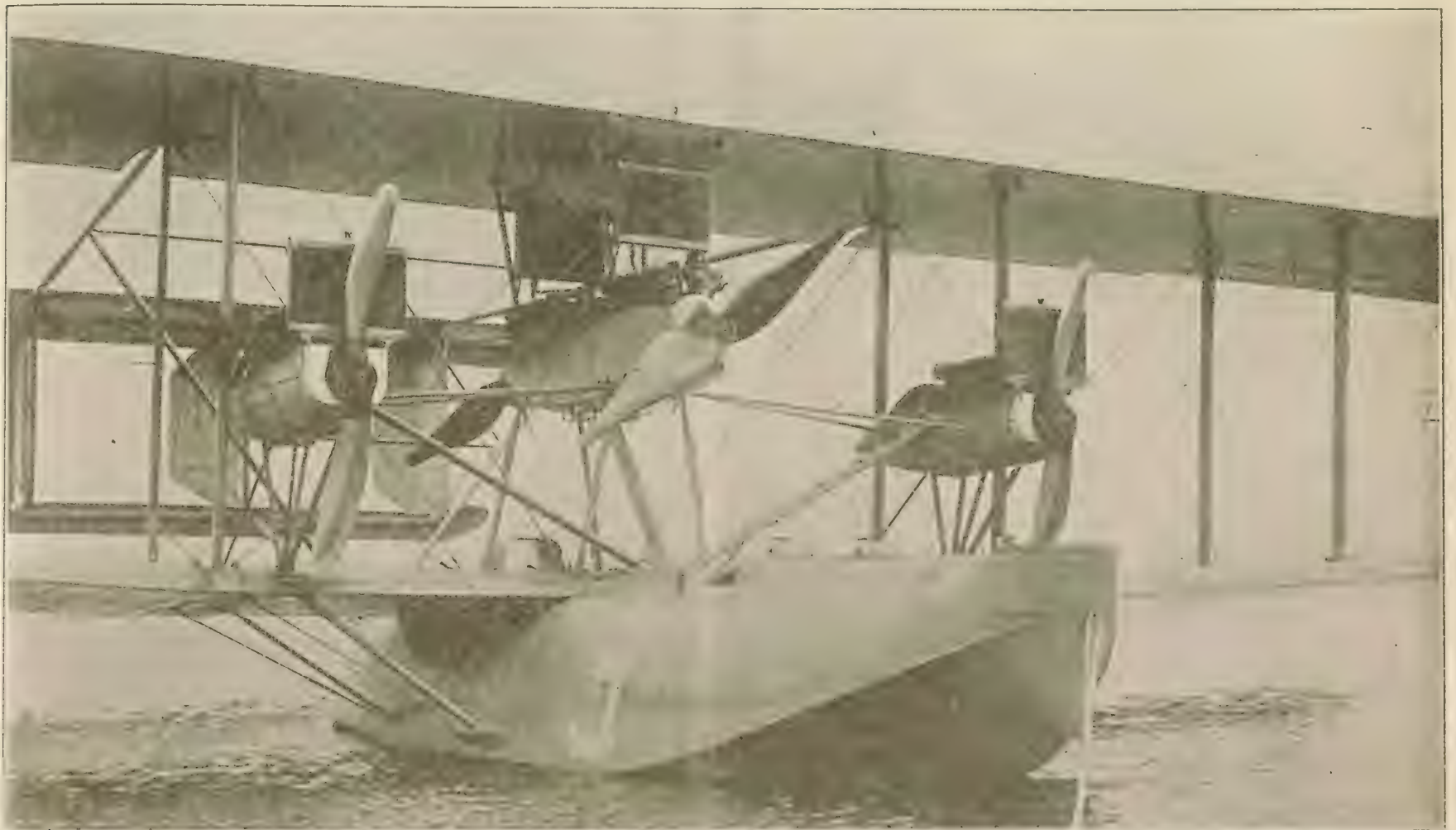
Close-up View of the NC-3 Now Ready for the Atlantic Flight. Two Types of Propellers are Shown. Those in the Center are Olmstead and the Others are Curtiss Types
